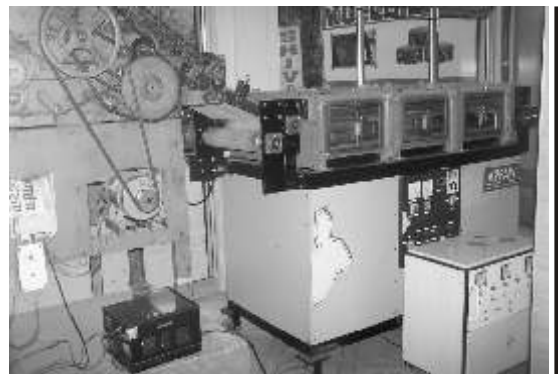
ALMOSPHERIC PRESSURE AIR PLASMA SYSTEM TO TREAT ANGORA WOOL
