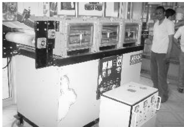
ALMOSPHERIC PRESSURE AIR PLASMA SYSTEM TO TREAT ANGORA WOOL
