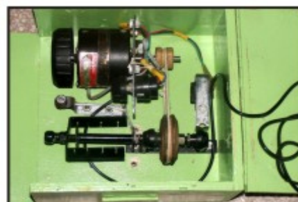
MECHANIZED SPINNING WHEEL DEVELOPED BY HIFEED
