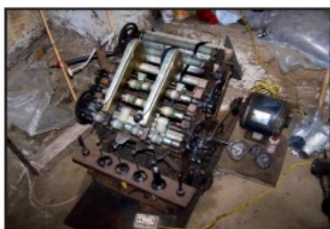
MECHANIZED AMBAR CHARKHA DEVELOPED BY HIFEED
